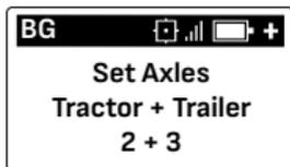
The number of axles needs to be selected using the Scrolling Up ↑ / Down ↓ buttons
